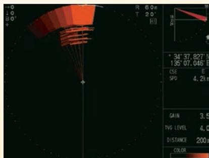
The Full-circle A-Scope mode shows the last detected echoes with one single color. The more opaque the color, the stronger the echo. The strength of an echo is clearly shown and it becomes easier to understand the nature of this echo.
