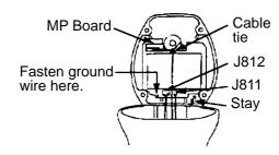
Figure 6-19 Antenna unit, cover opened
