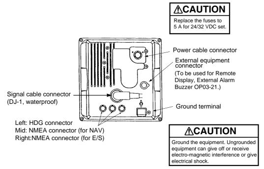
Figure 6-20 Connections on the display unit
