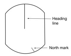
Figure 2-6 Heading line and north mark
