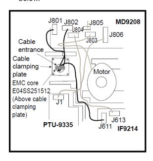
Figure 6-8 How to attach EMC core
