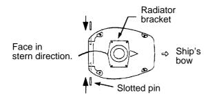
Figure 6-16 How to insert slot pins
