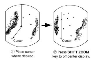
Figure 2-12 Shifting the picture
