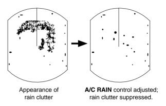
Figure 2-5 Effect of A/C RAIN
