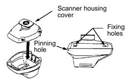
Figure 6-15 Fastening the antenna housing cover
