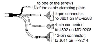
Figure 6-6 Signal cable, antenna unit side
