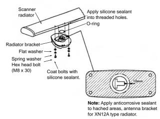
Figure 6-18 Fastening the radiator to the radiator bracket
