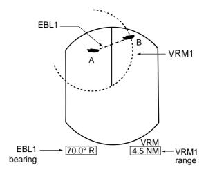
Figure 2-11 Measuring the range and bearing between two targets by using the offset EBL
