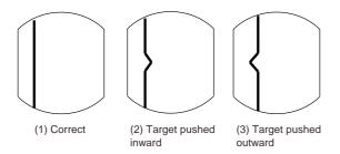
Figure 6-24 Examples of improper and correct sweep timing
