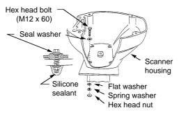
Figure 6-12 How to mount the antenna housing
