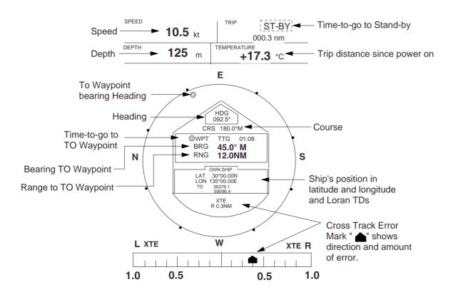
Figure 2-3 Typical navigation data display during stand-by
