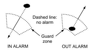
Figure 3-7 In and Out alarm
