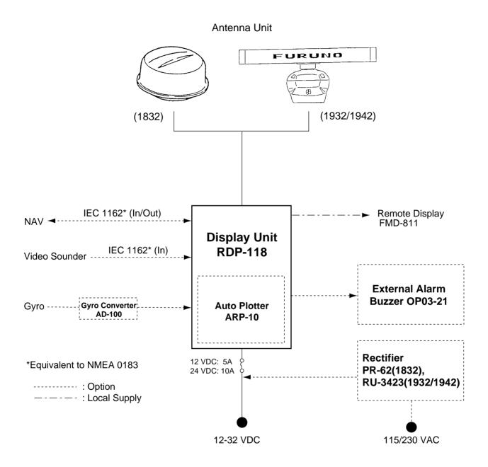
**Note:** Even though the display unit meets waterproof standard IPX-5, the connection of external buzzer, radar plotter and/or remote display can affect waterproofness. Watertight integrity cannot be guaranteed. When these modification has been done, the display unit should not be mounted where exposed.
