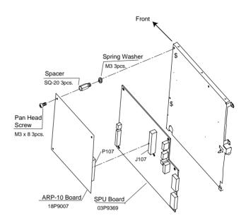
\$: Pull the front panel slightly to fix these screws.
