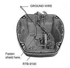
Figure 6-14 Connection in the antenna housing
