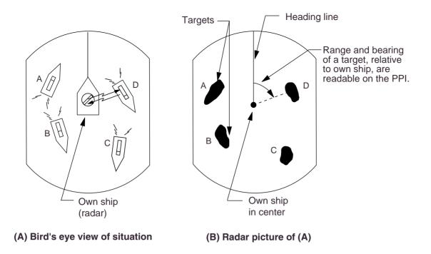
Figure 1-1 How radar works
