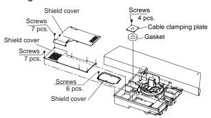
Figure 6-5 Antenna unit, inside view
