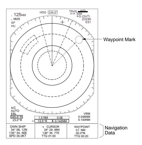
Figure 3-10 Typical navigation data display
